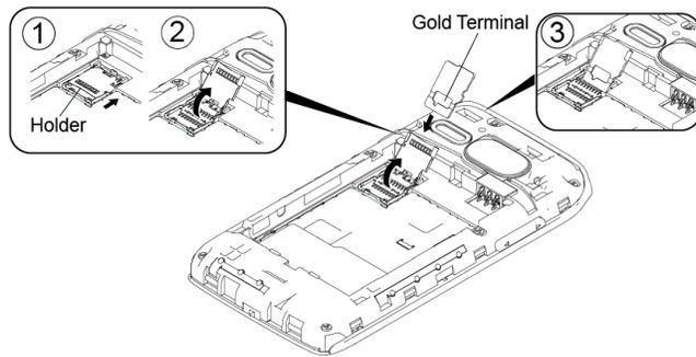
6. Replace the card holder and gently press it, and then slide the holder in the direction of arrow to lock it (④ and ⑤)
